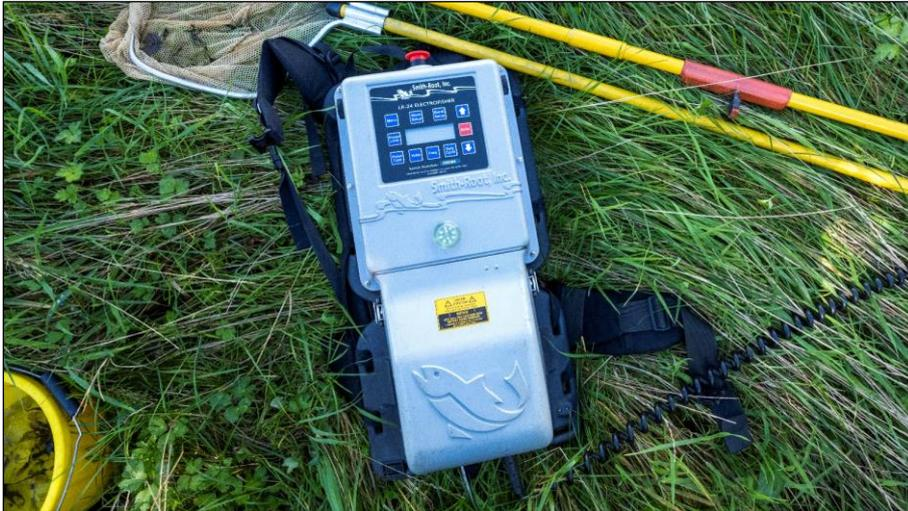
**Plate 1** The Smith-Root LR-24 back pack electrofishing unit used during the current survey.
